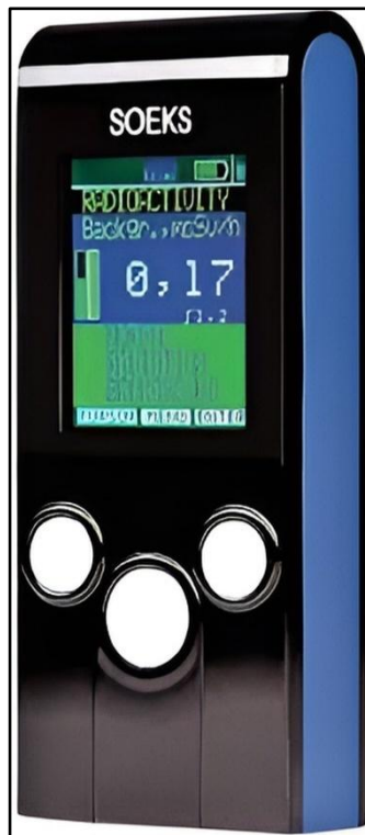
Fig.2. SOEKS 01M radiation detector (Germany Secondary Standard Dosimetry Laboratory Calibrated G.M. detector).
