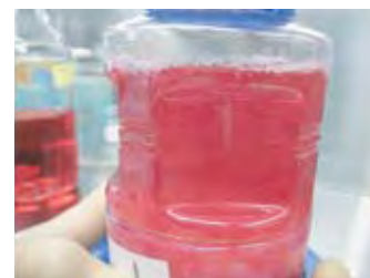
Matrix dissolved and cell mass dislodged from the matrix for harvest after cell culture.
