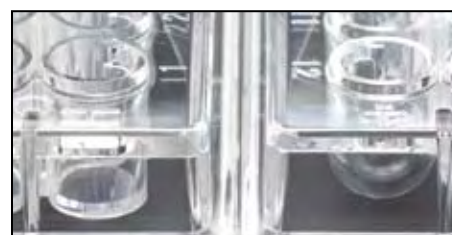
Close-up view of flat bottom (left) and round bottom (right).
